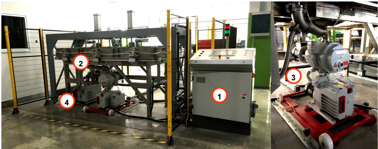
1. Control Station 2. Vacuum Test Chamber 3. Vacuum Pump and Blower 4. Helium Mass-Spectrometer
